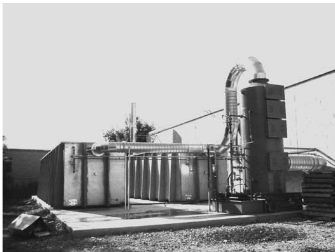
Fig. 3 Commercial 7,500-cfm-capacity biofilter system at a printed circuit board manufacturing facility (Toronto, Canada). One unit is filled with the wood media and the other with a manufactured inorganic medium
